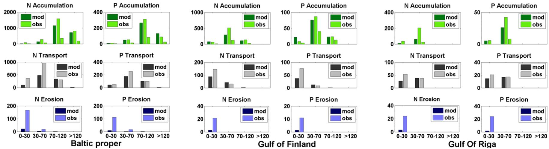
Modelled nitrogen and phosphorus content (kton) at the different bottom types and different depth intervals compared to estimations based on observations.
